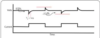
Typical transient response specification for a switch-mode programmable DC power supply:
